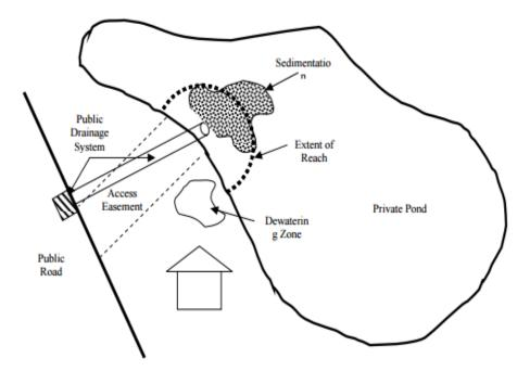
Figure 1. Typical outfall sediment removal activity components.
