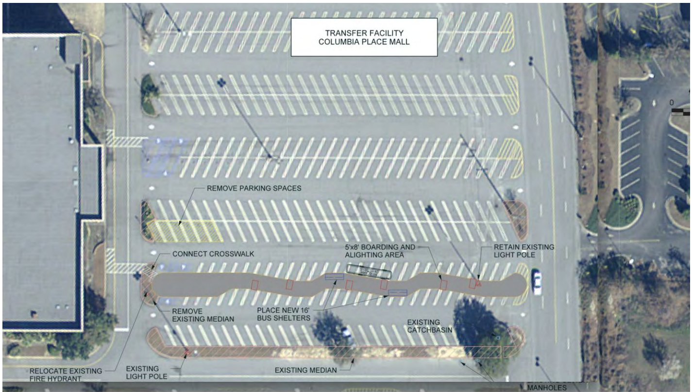
Image 3. Draft sketch of the proposed Northeast Connection Protection Zone. Sketch was made for illustration purposes only, it is not a final design.
