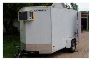
*Refrigeration trailer using A/C system with CoolBot* technology. Credit: EverGood Farm
