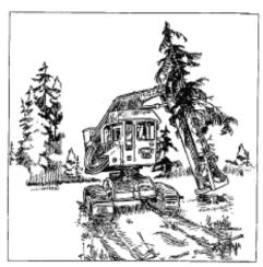
Figure 5. Feller-buncher.
